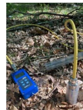
Tubes + sonde TDR Eau -> 1m40
